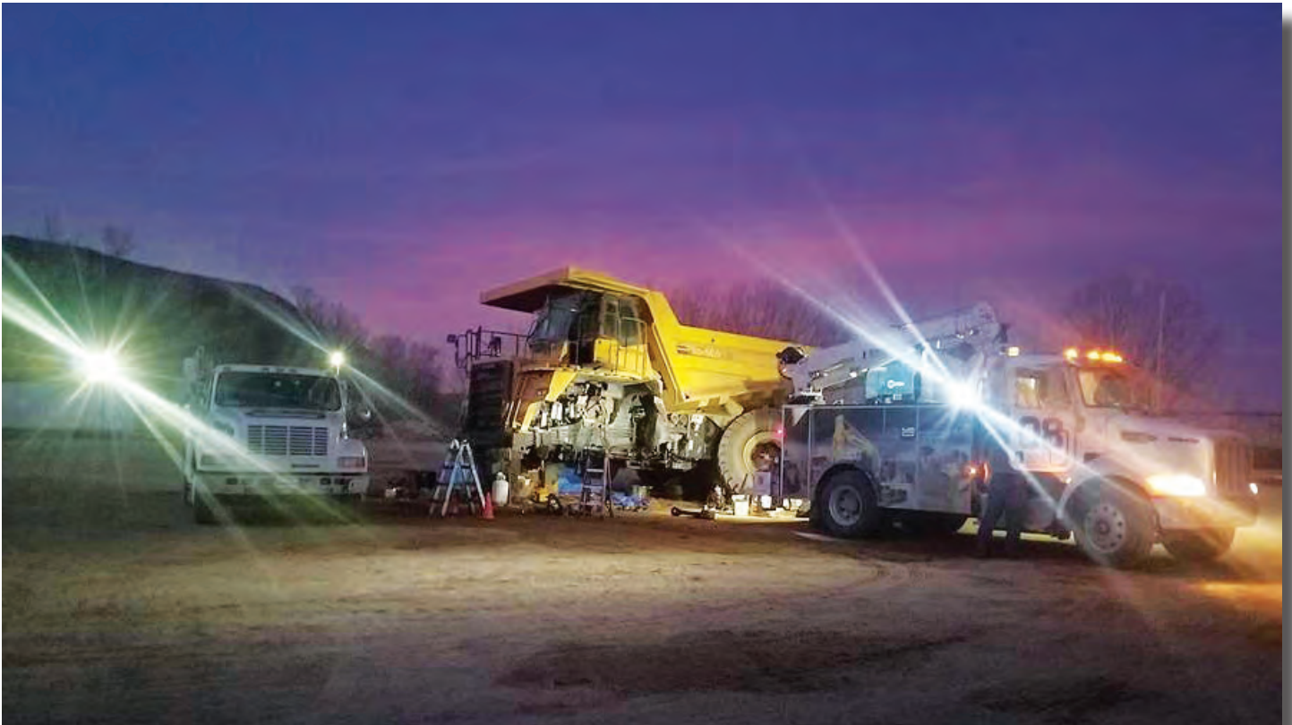
Field Technicians Steve Richard and John Schoenenberger service a Komatsu HD465-7EO with 27,000 hours at the APAC Quartzite Quarry in Lincoln, KS.
